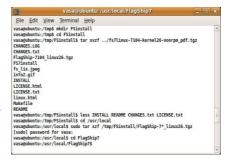
The following installation sequence requires log-in as super user (su) or root. An alternative (used e.g. in Ubuntu) is the restricted **sudo** command:
